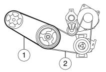
1. Short drivebelt is on first pulley groove closest to engine (except vehicles with electric power assisted steering).
